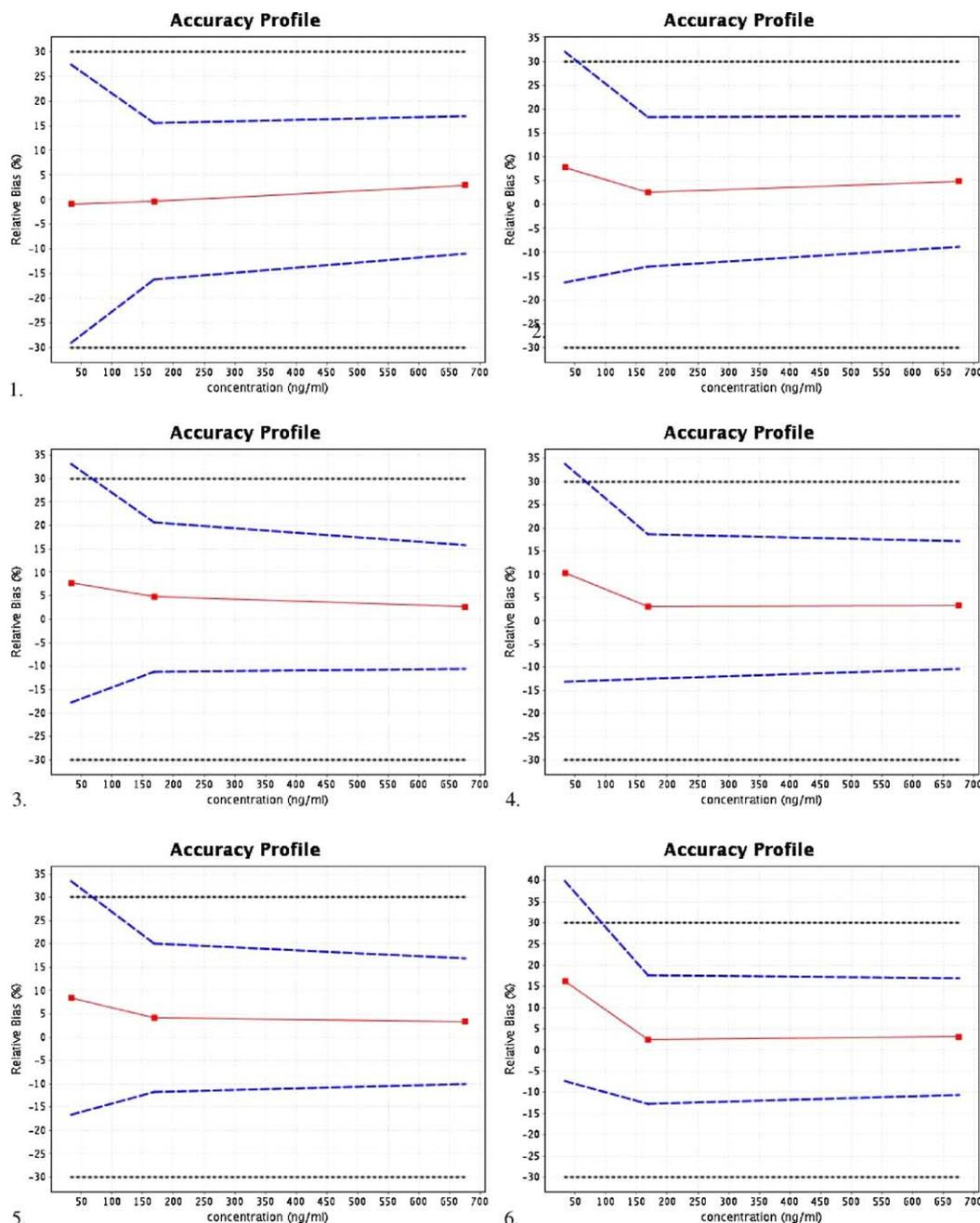
Fig. 4. Accuracy profiles of CPA in epidermis using (1) linear regression through 0 fitted with the highest concentration level only, (2) weighted linear regression model, (3) quadratic regression, (4) linear regression model after square root transformation, (5) linear regression model after logarithm transformation, (6) linear regression model.
