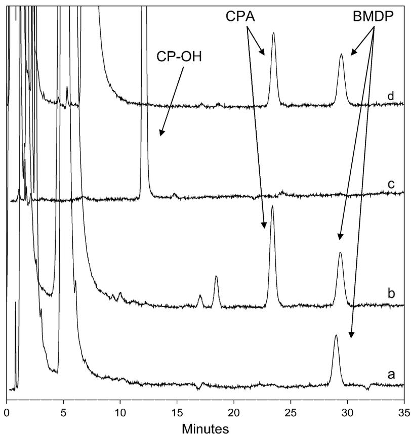
Fig. 2. Chromatograms of epidermis extracted with methanol and of a CP-OH solution. (a) Sample spiked with BMDP (1667 ng/ml). (b) Sample spiked with CPA (33 ng/ml) and BMDP (1667 ng/ml). (c) Solution of CP-OH (500 ng/ml). (d) Sample obtained from diffusion tests through the skin. Analytical column: Lichrospher RP-18 (250 mm  $\times$  4.0 mm, i.d.); HPLC mobile phase: acetonitrile/water (40:60 (v/v)).
