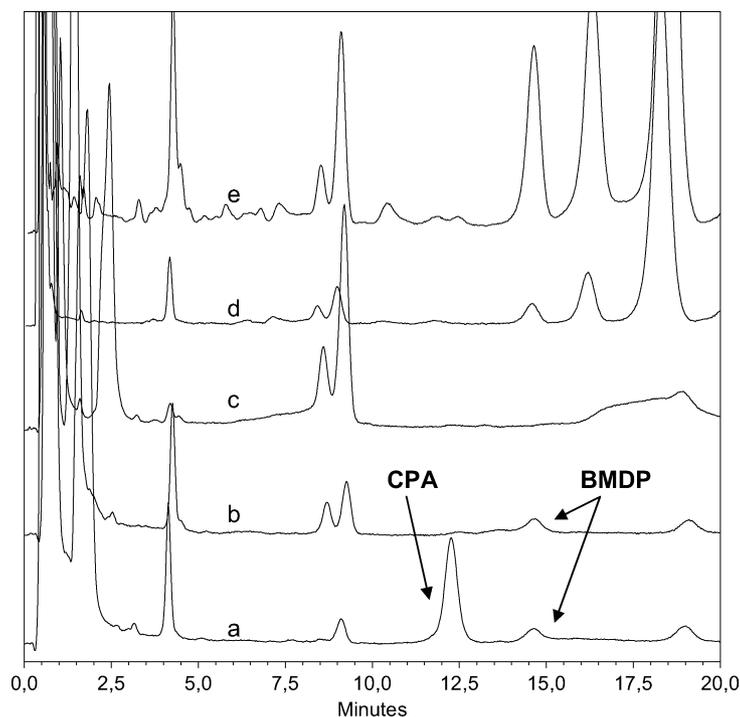
Fig. 1. Chromatograms of dermis extracts. (a) Dermis extracted with methanol and spiked with CPA (333 ng/ml) and BMDP (667 ng/ml). (b) Dermis extracted with methanol and spiked with BMDP (667 ng/ml). (c) Dermis extracted with acetonitrile. (d) Dermis extracted with hexane. (e) Dermis extracted with dichloromethane. Analytical column: Lichrospher RP-18 (125 mm × 4.0 mm, i.d.). HPLC mobile phase: acetonitrile/water (40:60 (v/v)).
